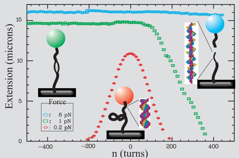
With an impressive dynamics of force (0.01 pN to 100 pN, depending on the bead size), **PicoTwist** fits a large variety of biological applications. However, the main feature of **PicoTwist** is its ability to induce a torque into the substrate of interest, and thus to achieve a perfect control of its mechanical state.
