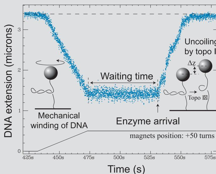
Besides Topoisomerases, magnetic tweezers apparatus like **Picotwist** have been shown to be extremely useful to study fundamental classes of enzymes, such as Helicases, Restriction enzymes, and Polymerases at the molecular level.
