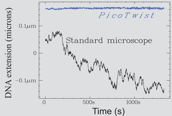
**PicoTwist** has been designed to ensure an optimal mechanical stability. Low drift is a critical requirement to achieve the detection of protein/DNA interactions at the scale of the nanometer.
